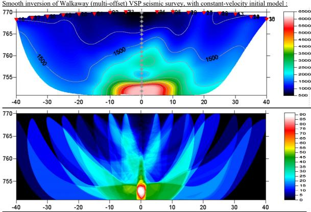
Borehole *station spacing* 1m, shot interval 5m, 200 WET iterations with default WET parameters and settings. Top: velocity tomogram in m/s. Bottom: first break energy and wavepath coverage, in paths/grid cell.
