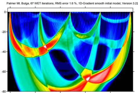
Fig. 14 : WET wavepath coverage shown with Fig. 13.
