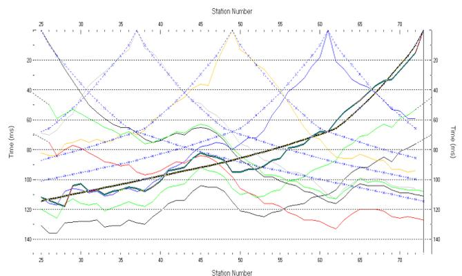
Fig. 4 : *Refractor|Shot breaks* display. Browse traveltimes curves with F7/F8. Solid colored curves are picked times, dashed blue curves are modeled times, for starting model shown in Fig. 5 . RMS error is 7.1%.
