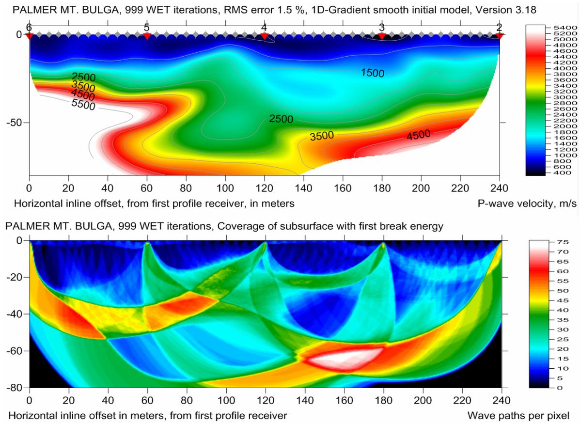
Fig. 2 Smooth 2D inversion version 3.18, 999 WET iterations (Schuster and Quintus-Bosz 1993), default parameters. Top: velocity. Bottom: wave path coverage. Note strong lateral velocity variation and velocity inversions in overburden. There are no laterally continuous refractors. Far-offset shots not regarded. We recommend to record shots with overlapping receiver spreads.
