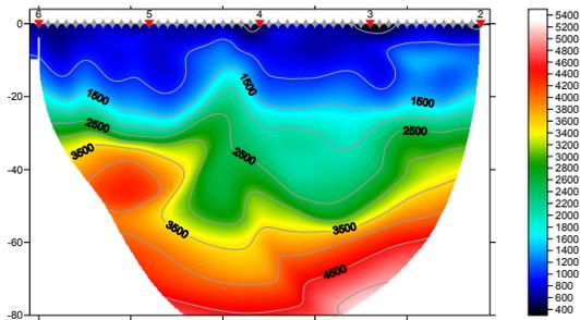
Fig. 6 : Velocity tomogram with Smooth inversion, 20 WET iterations, default settings, wavepath width 5.5%. RMS error is 2%. Starting model is Fig. 5.
