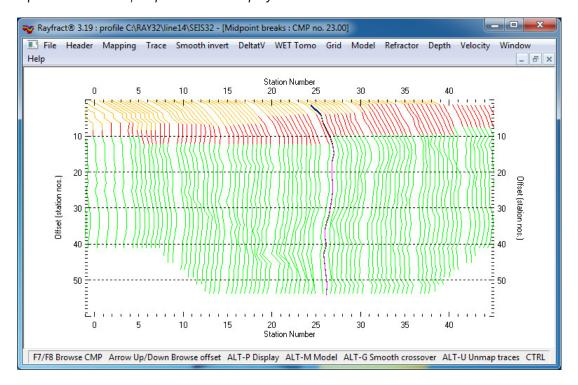
Browse CMP sorted traveltime curves with F7/F8 function keys. Browse offset along one curve with Arrow Up/Arrow down keys. The status bar will show local apparent velocity etc.
