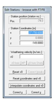
By convention elevation of *borehole receiver stations* is negative, relative to elevation 0 at topography. As a consequence *station numbers* are negative too. **Station numbers are computed by dividing the station elevation with** *Station spacing* **specified in** *Header***|***Profile***.**
