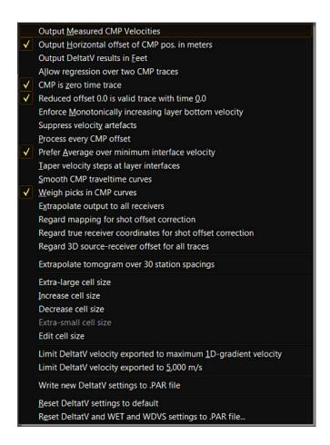
If the Smooth inversion interpretation shows at least some degree of quasi-horizontal subsurface layering you may optionally run pseudo-2D DeltatV based WET inversion . **To start the automated version of our pseudo-2D DeltatV inversion select** *DeltatV|Automatic DeltatV and WET inversion.*
