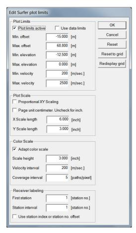
Click button Reset to grid reset to offset/elevation/velocity range to selected profile VELOITXY.GRD tomogram in subdirectories ...\GRADTOMO, ...\LAYRTOMO, ...\TOMO or ...\HOLETOMO.
