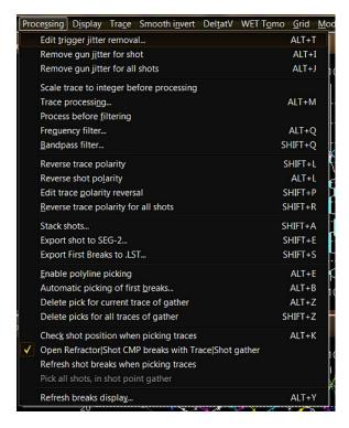
Since version 3.20, above *trace display* settings and following *trace filtering* and *trace processing* settings are stored separately in your profile database for each gather type (shotsorted, midpoint-sorted, offset-sorted, shotpoint-sorted, receiver-sorted). Also, these settings are restored whenever you reopen this profile database via *File menu*, and when you reopen these gather type displays with *Trace menu*.
