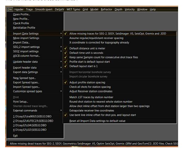
Open Profile... Opens an existing database. Select SEIS32.DBD in profile
