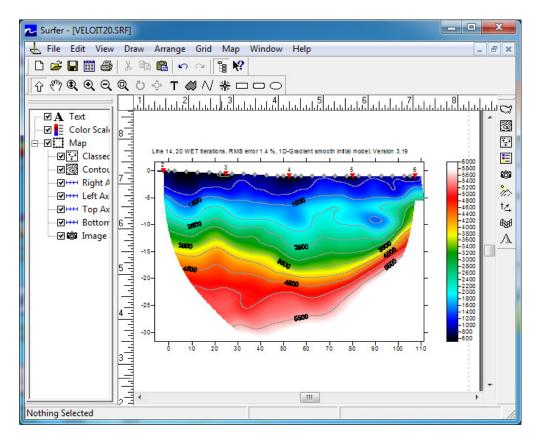
Use CTRL+TAB key combination in Surfer®, to view WET wavepath coverage plot:
