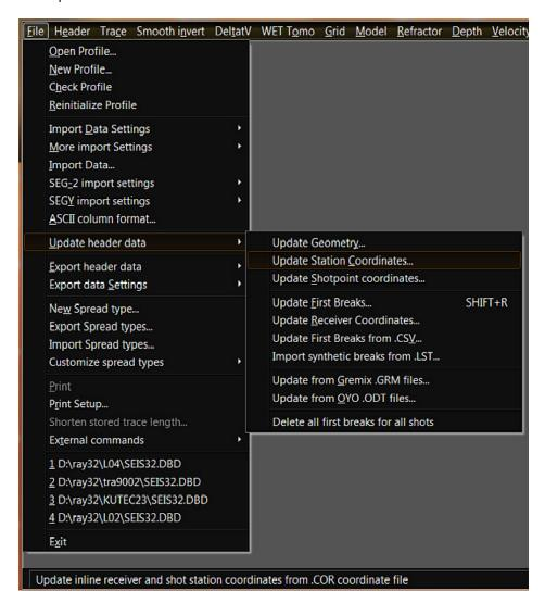
Spread types are stored in the reference database (directory \RAY32\REF, files SEISRF32.\*), and not in the individual profile databases. So any custom spread type defined earlier is available for all profile databases. After installing an updated version of our software, you may want to reimport your custom spread types stored in \RAY32\REF\MYSPREAD.SPR or \RAY32\
