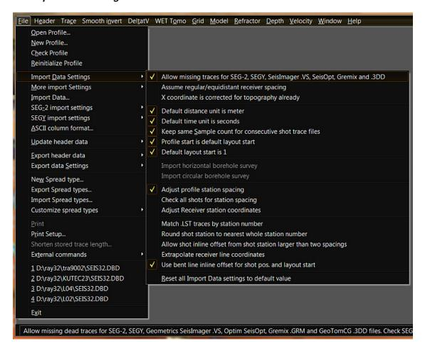
**Allow missing traces for SEG-2, SEGY, SeisImager, SeisOpt, Gremix and .3DD**Allow missing dead traces, for Geometrics SeisImager, Optim SeisOpt, Interpex Gremix, GeoTomCG .3DD and Geogiga .TTX files
