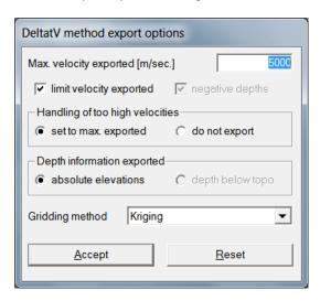
Edit parameters determining the format of the ASCII output file DELTATV.TXT, generated at the end of the DeltatV inversion :
