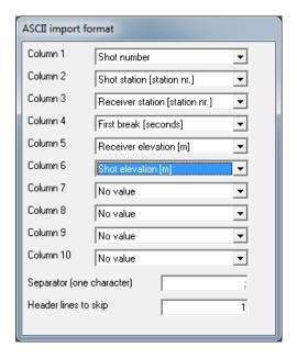
Once you have done this, generate ASCII.ASC files with third-party software e.g. Microsoft Excel or W\_GeoSoft WinSism. Then import these ASCII.ASC files with *File/Import Data...* and *Import data type ASCII column format*.
