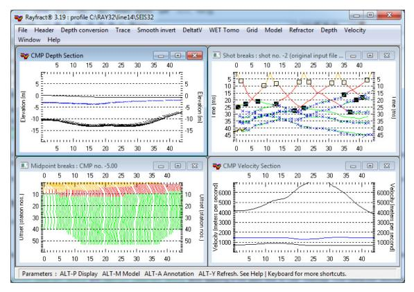
The accuracy of refractor depths and velocities obtained is limited in case of strong refractor curvature. Select *Velocity/CMP Refraction* to display corresponding velocities.
