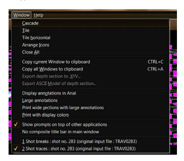
When displaying sections on screen, you may lay out up to three sections adjusted vertically and displayed below each other by selecting *Windows/Tile horizontally*. Be careful to specify the same profile section limits for all three sections. These limits may be specified in the *Display parameters dialog* for each section (ALT+P).
