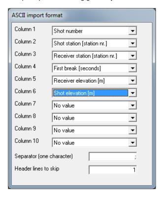
Specify the value separator in edit field **Separator**. The default separator is a semicolon (;). Another frequently used separator is a comma (,), as used by Microsoft Excel® when generating .CSV comma-separated value files.
