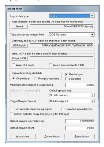
You need to check Batch import to enable batch import with .HDR file selected above.
