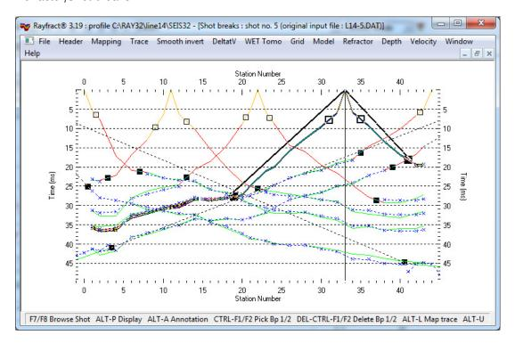
We split one travel time curve (forward or reverse shooting direction) into two or three segments or branches with *branch points* based on apparent velocity or dip of curve segment in *Refractor/Shot breaks display*.
